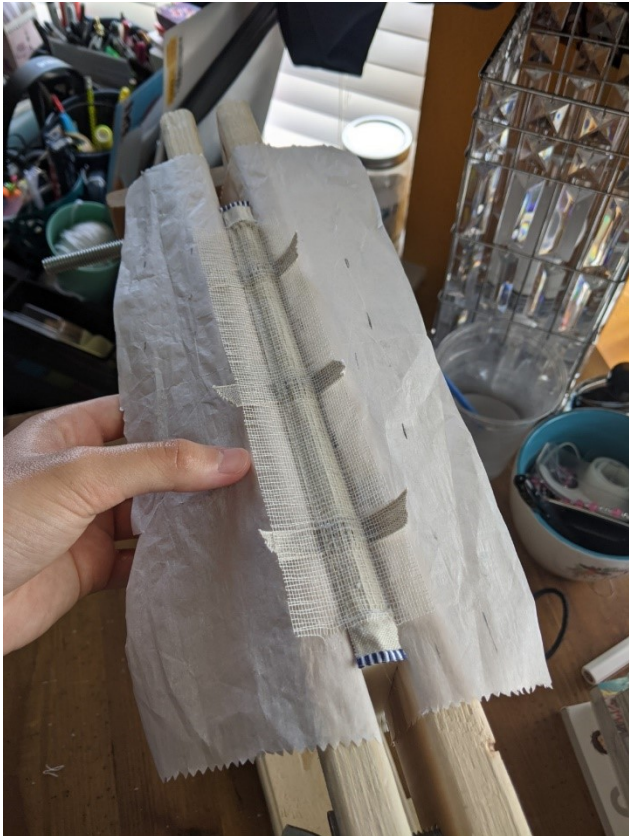
Second round of glue on the spine, this time with mull and headbands
