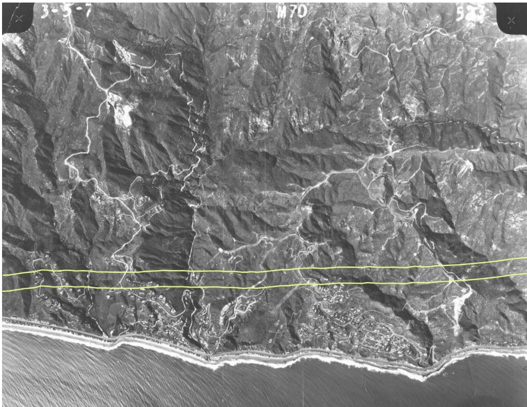
FIGURE 10. Example of a high resolution aerial photograph of the Malibu coastline showing Big Rock Mesa and southern Las Flores Canyon, with the inferred trace of the Malibu Coast Fault (Yerkes and Wentworth, 1965) bracketed between the yellow lines.
