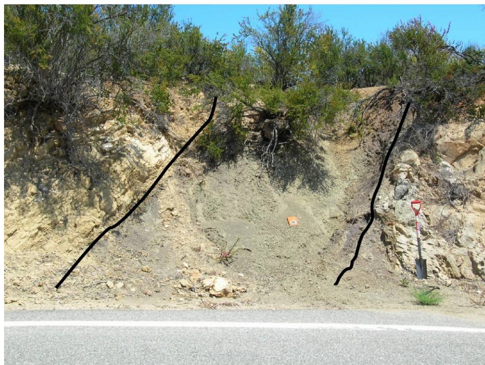
FIGURE 18. Fault at site B, an uninterpreted photograph at top. The same photo below with fault interpretation. Black lines indicate the edge of the fault zone. Note shovel for scale.
