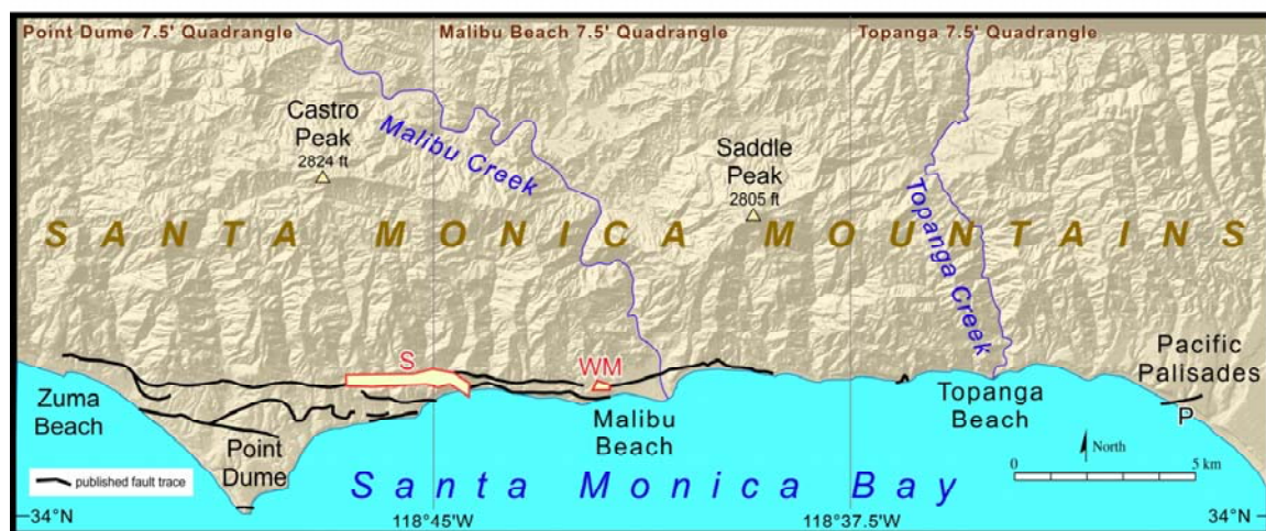
FIGURE 2. Elements of the Malibu Coast Fault Zone along the southern edge of the central Santa Monica Mountains. The only strands of this fault zone that are considered “active” by the criteria of the Alquist-Priolo Act are the Solstice strand (S) and the Winter Mesa strand (WM), whose study-zone boundaries are outlined in red. The Potrero Fault (P) displays 47 meters of vertical displacement during the last 124,000 years (Hill, 1979; LaJoie and others, 1979).
