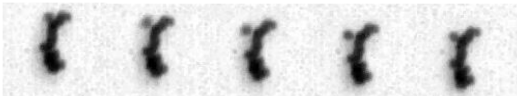
FIGURE 3. Sequence of consecutive images showing a single monomer at the upper left which is not physically attached to the aggregate but appears to be electrostatically bound ( \Delta t = 3.33 \times 10^{-4}\text{s} ).
