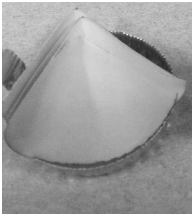
Figure A2. Filter paper used for a scute that was predigested. This modification showed improved results in that with the exception of the very tip, no scute residue was visual.
