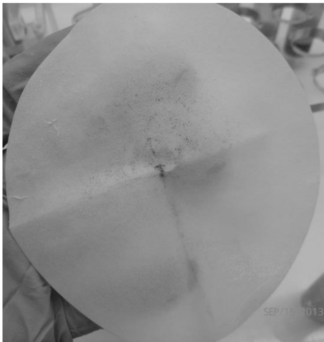
Figure A1. Practice scute residue left around the center of the filter paper. This visualization demanded for a modification in the digestion method EPA 3050B.
