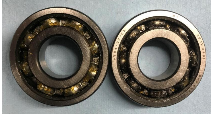
Figure 1.8. EDM discharges burn and degrade the bearing lubricant (right) as can be seen here compared to a bearing with new lubricant (left).
