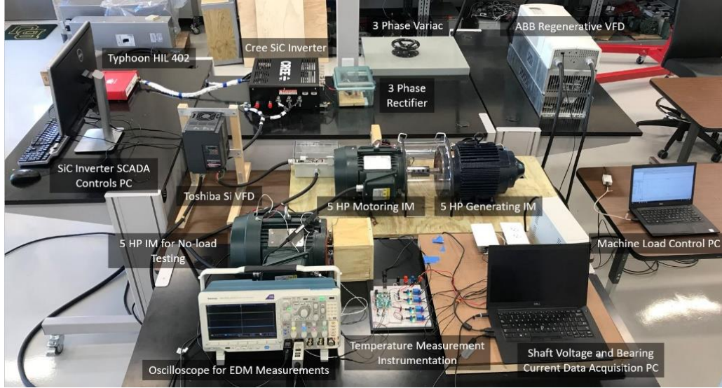
Figure 2.1. Machine testbed used for the characterization of CM voltages, shaft voltages, and EDM bearing currents due to Si and SiC PWM inverters.
