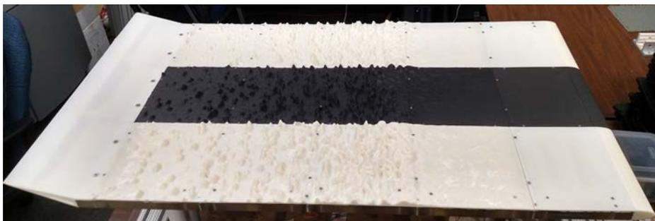
Figure 3.2: Full Plastic Manufactured Unwrapped Surface for 113012.04 Case [10]
