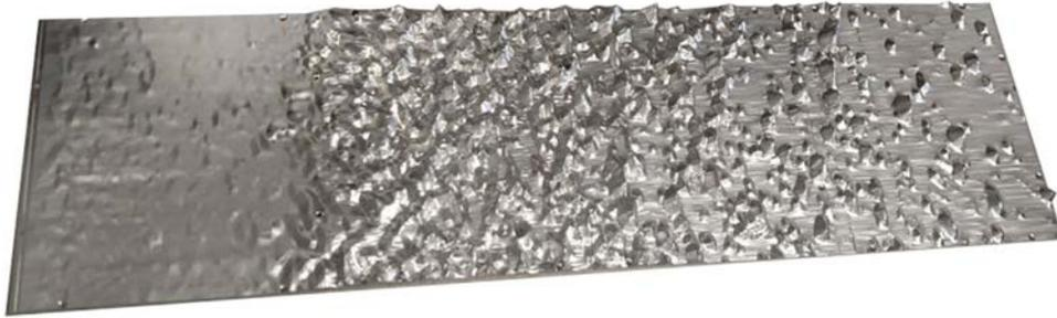
Figure 3.1: Unpainted aluminum heated section for 113012.04 Case [10]
