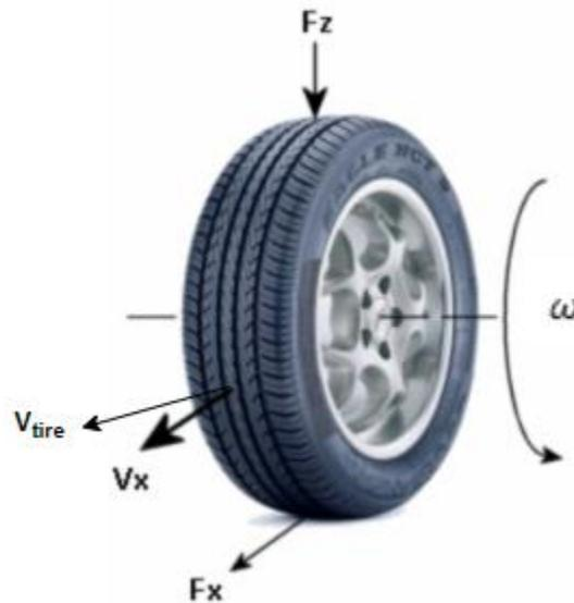
Figure 2.7. Speed and forces in the tire-road contact patch area [39].
