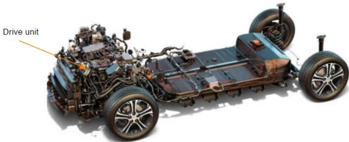
Figure 2.1. Chevrolet Bolt, Single Speed Direct Drive Unit [31].
