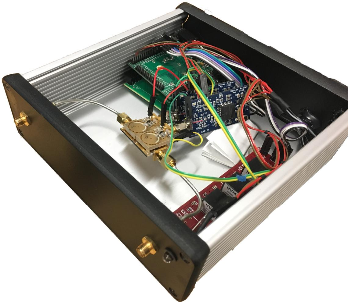
Figure 6.1. First-generation evanescent-mode cavity tuner with piezo actuators developed by Purdue University [25]. © 2019, IEEE.
