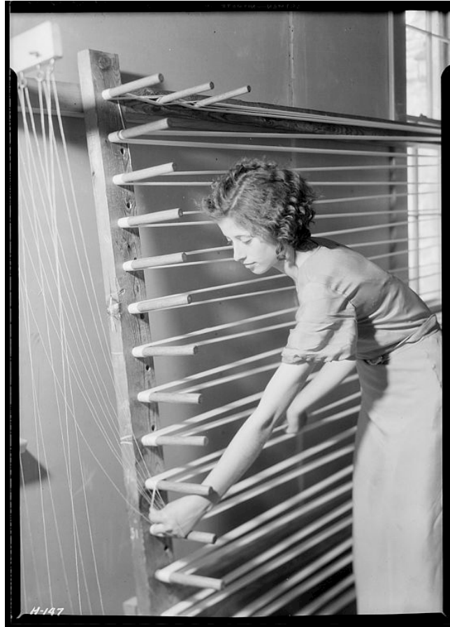
Fig. 7.36: 1930's Device for Preparing Warp for Weaving, from The U.S. National Archives. No Known Copyright Restrictions. 80
