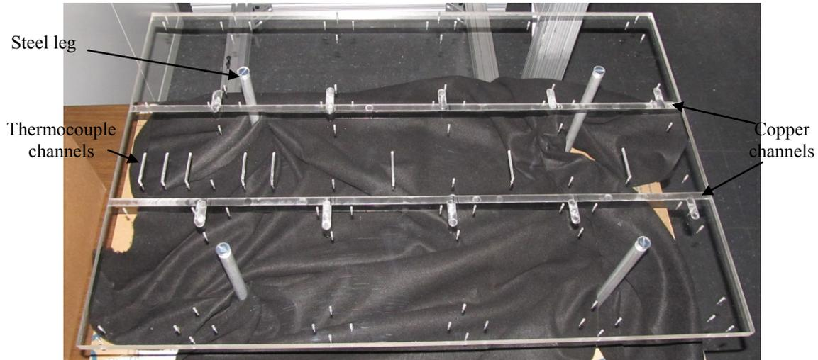
Figure 3.5: Plexiglas test plate after initial machining
