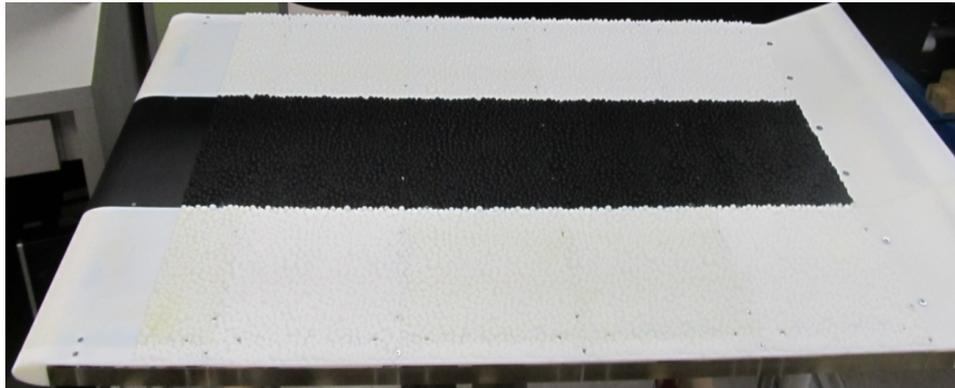
(b) Printed surface installed on test plate
