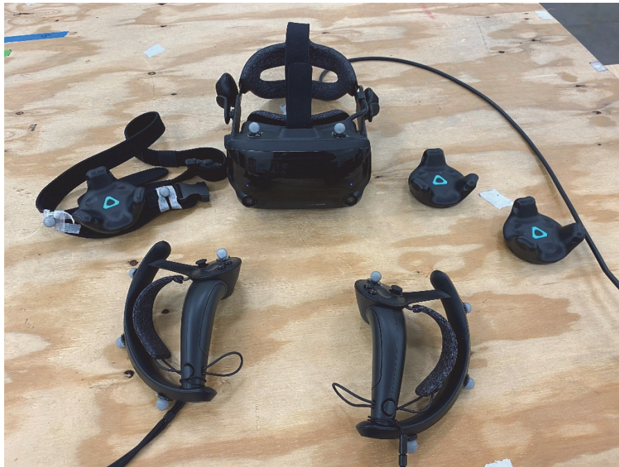
Figure 1.1: Valve Index HMD, Controllers, and Vive Trackers
