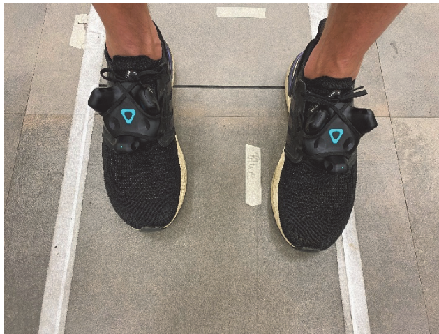
Figure 3.3: Vive Trackers secured in the laces of the user's shoes
