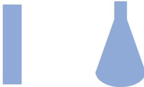
Figure 3.3. Top view of (left) rectangular matching stub and (right) radial matching stub.
