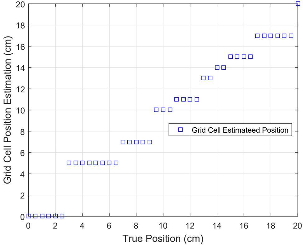
Figure 3.3 Grid Cell Estimation vs Truth: When multiple grid cells are fired at the same locations, they each provide their own phase. This means phases provided by different grid cells, when combined, represents location on the axis as described in (3.2). This figure shows what location a grid cell encodes to (on the y-axis) at every .5 cm along the axis with 6 grid cells the lattices sizes of 5, 7, 11, 13, 17, and 23 cm as used to provide the results presented in Chapter 4.
