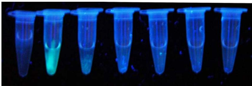
Figure 11.7: Salt concentration effect on GH Sepharose 4B stability. From left to right: Negative control, positive control, 0, 0.1, 0.25, 0.5, and 1 M NaCl
