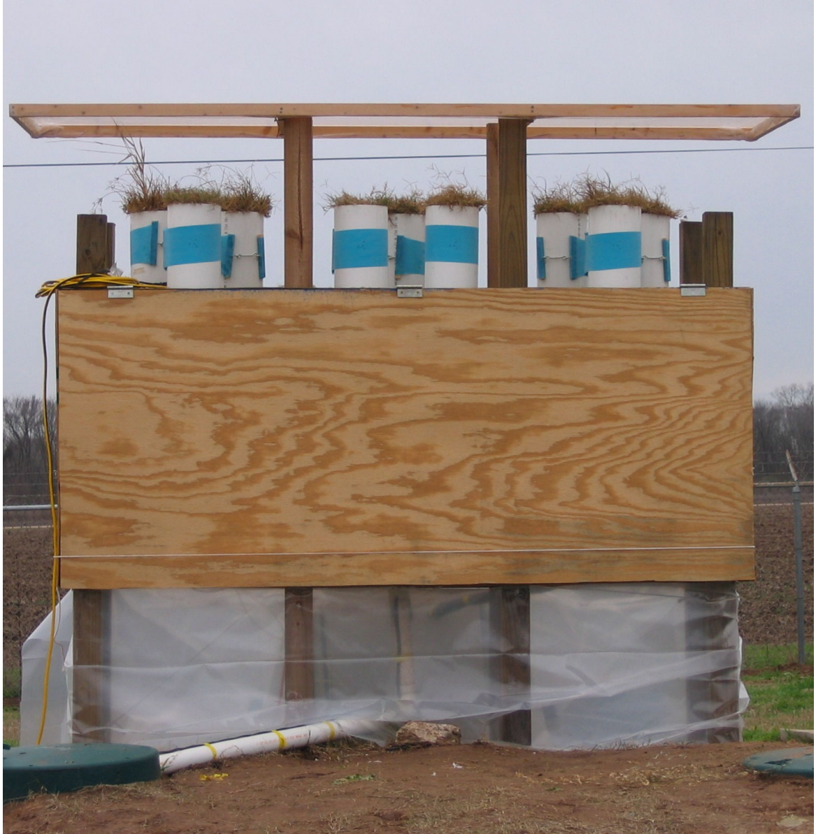
Figure 5. Soil column apparatus showing top of the septic tank (green riser) from which effluent was pumped, the heated wooden enclosure helped prevent freezing and maintain fairly consistent temperature at “depth” and the rain shield above the columns.
