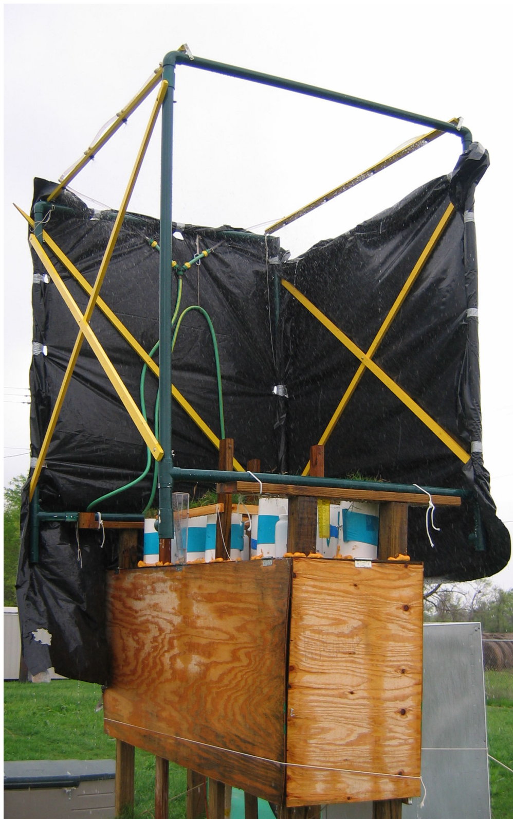
Figure 6. Soil columns during a rain event simulation showing the rainulator, rain gauges and protective plastic windshield to help maintain even rain distribution
