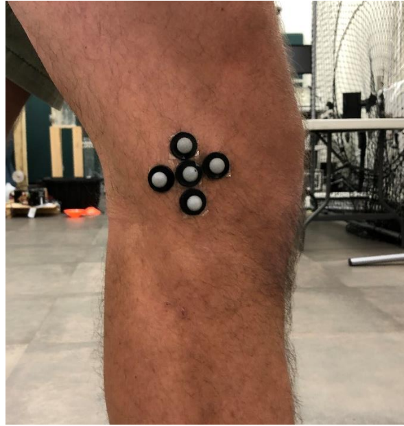
Fig 4.3: Kinematic trials knee marker configuration.
