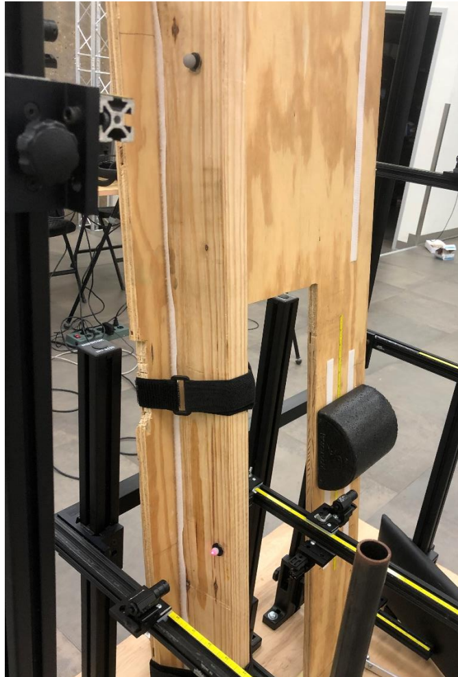
Fig 3.6: Markers placed and laser projection on rigid body.
