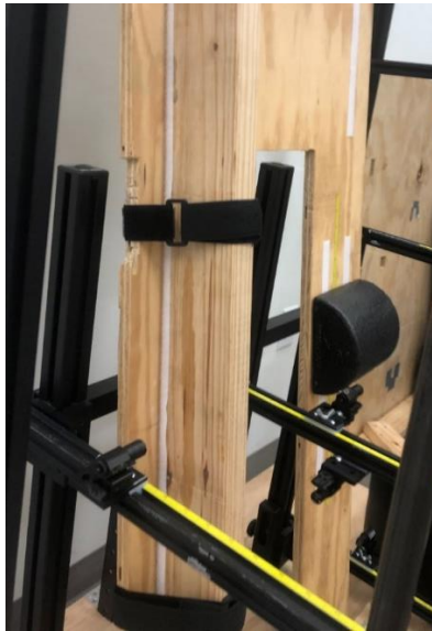
Fig 3.4: Rigid body attachment for laser projection trial.
