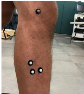
Fig 4.1: Reference markers placed on tibial segment.
