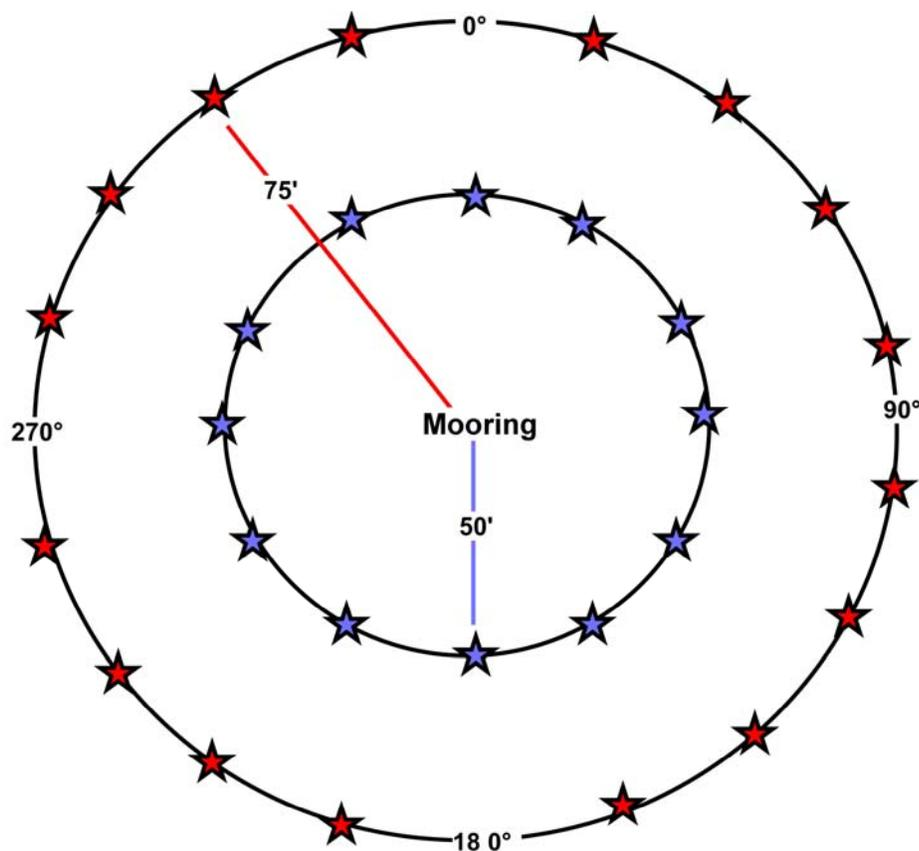
Figure 12. Diagram depicting the method used for the bathymetric surveys at the Red Buoy Patch Reef at a 50 and 75 foot radii. This method has essentially remained consistent since the first survey in 1974. Red and blue stars indicate degree positions where depth was measured corresponding to 20° increments; 20°, 40°, 60°, 80°, etc. for the 75 foot radius and 20° for the 50 foot radius.
