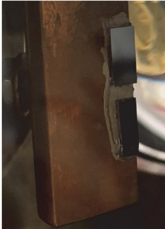
Figure 3.6. Both samples mounted on the copper block with silver paint. The top sample did not have graphene, while the bottom sample had a graphene top contact.
