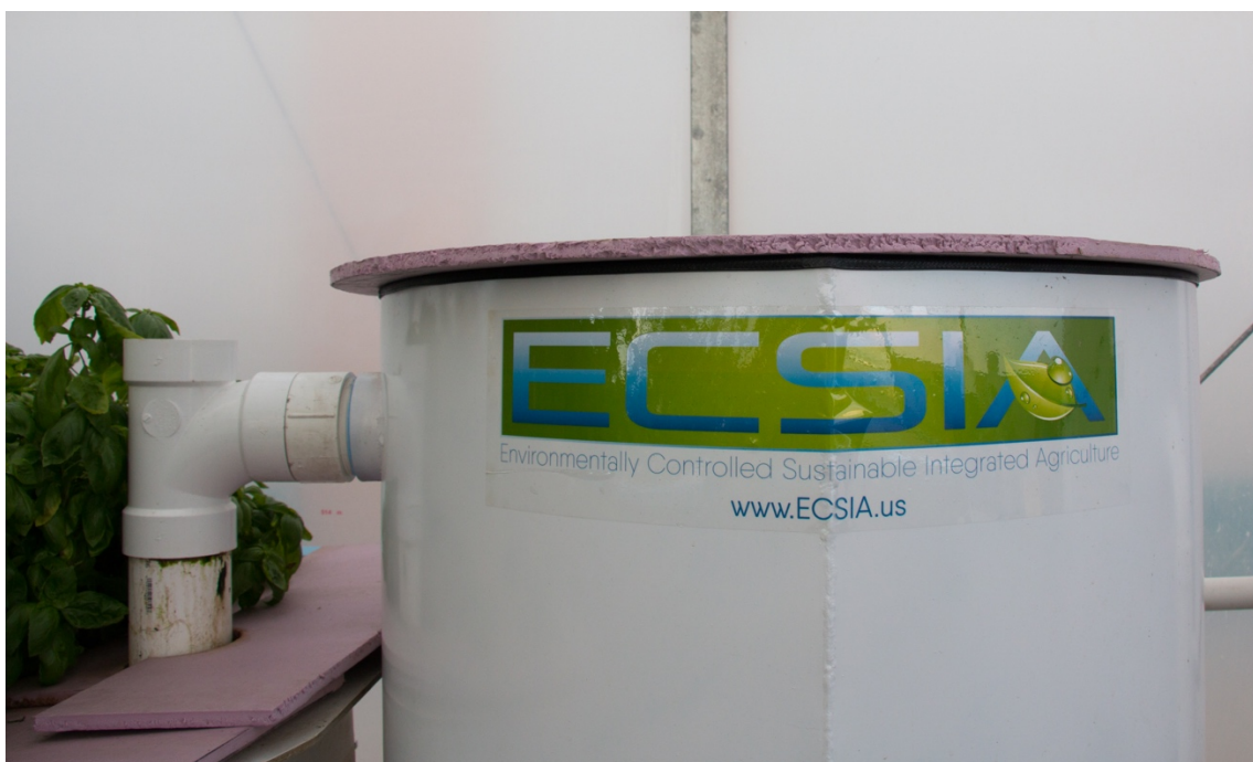
Figure 29: The fish tank holds about 280 hybrid striped bass. The ammonia waste produced by the bass is converted to nitrate by the bacteria grown throughout the system.
