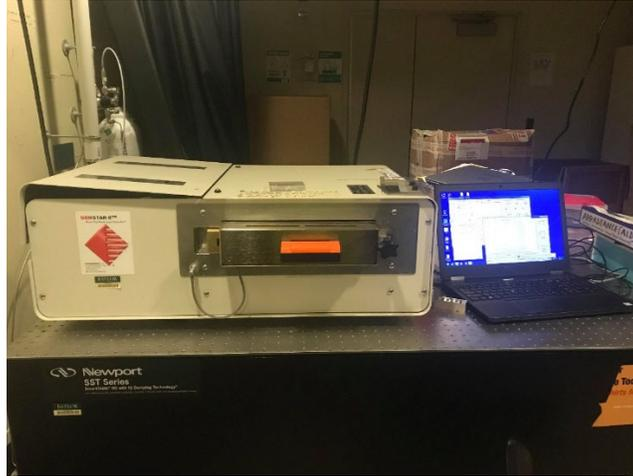
Figure 3.5 The ALD machine situated at Lee nano-optics lab at Baylor science building.
