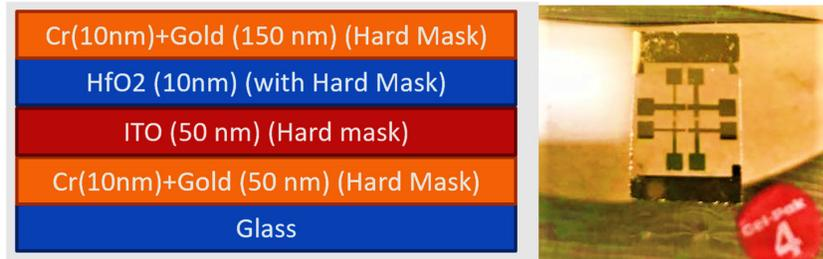
Figure 3.7 (Left) Schematic diagram of sample and (right) the optical image of the sample.
