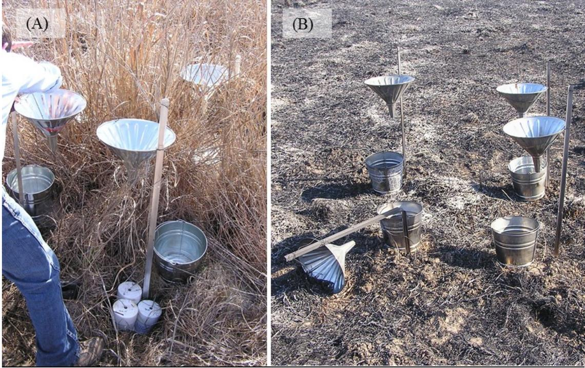
Figure 6. Reynolds Creek Sampling apparatus. (A), Before the burn; (B), After the burn. Note one of the poles had melted partway up during the burn and is lying on the ground.
