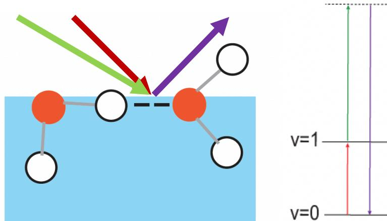
Figure 1.2. Schematic depicting the SFG generation from IR and visible beam overlap on the interface of water (left) and an energy diagram of SFG (right).
