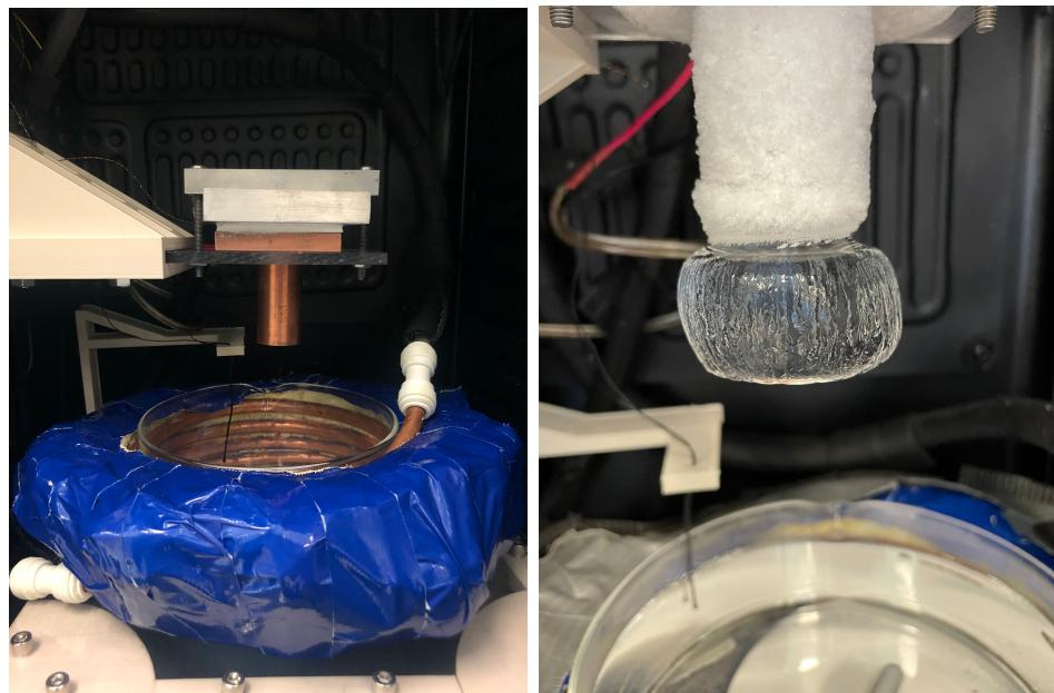
Figure 2.1. Ice growth apparatus including a crystallizing dish, surrounded by copper tubing with chiller solution to maintain ice bath temperature, including the copper pin (a). An ice growth prior to harvesting (b).
