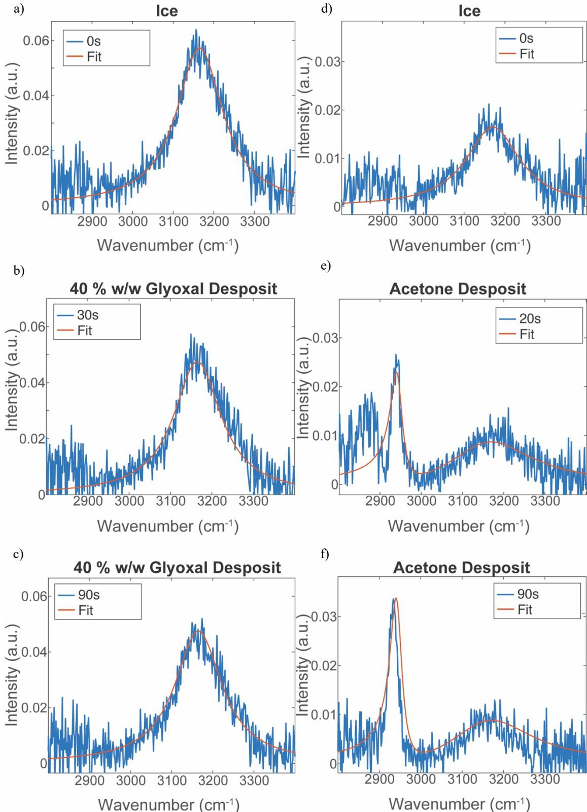
Figure 3.4. SFG spectra of glyoxal vapor deposition on ice for 0s (a), 30s, (b), and 90s (c) and acetone vapor deposition on ice for 0s (d), 20s (e), and 90s (f) in the CH stretch region (blue) with fitting (red).
