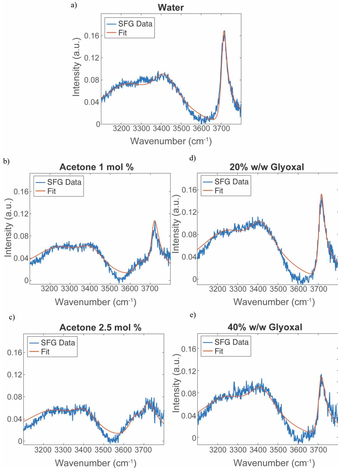
Figure 3.2. SFG spectra of water (a), acetone 1 mol % (b), acetone 2.5 mol % (c), glyoxal 20 % w/w (d), and glyoxal 40 % w/w (e), solutions in the free OH region (blue) with fitting (red).
