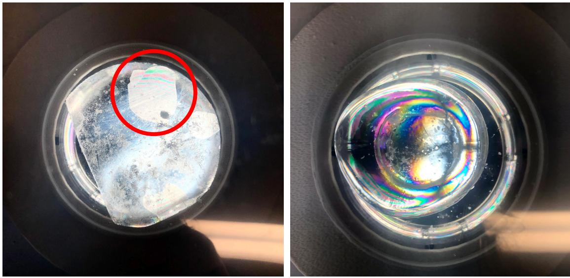
Figure 2.2. Images of ice boules under cross polarizers of polycrystalline ice (left) with a domain circled in red and single crystalline ice (right).
