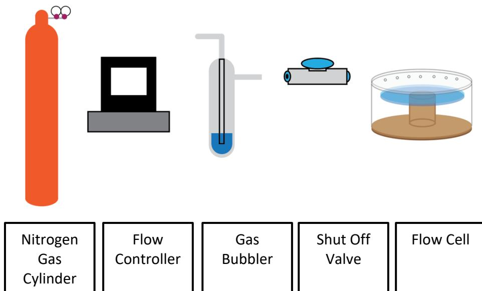
Figure 2.5. Schematic diagram of the nitrogen flow set up.
