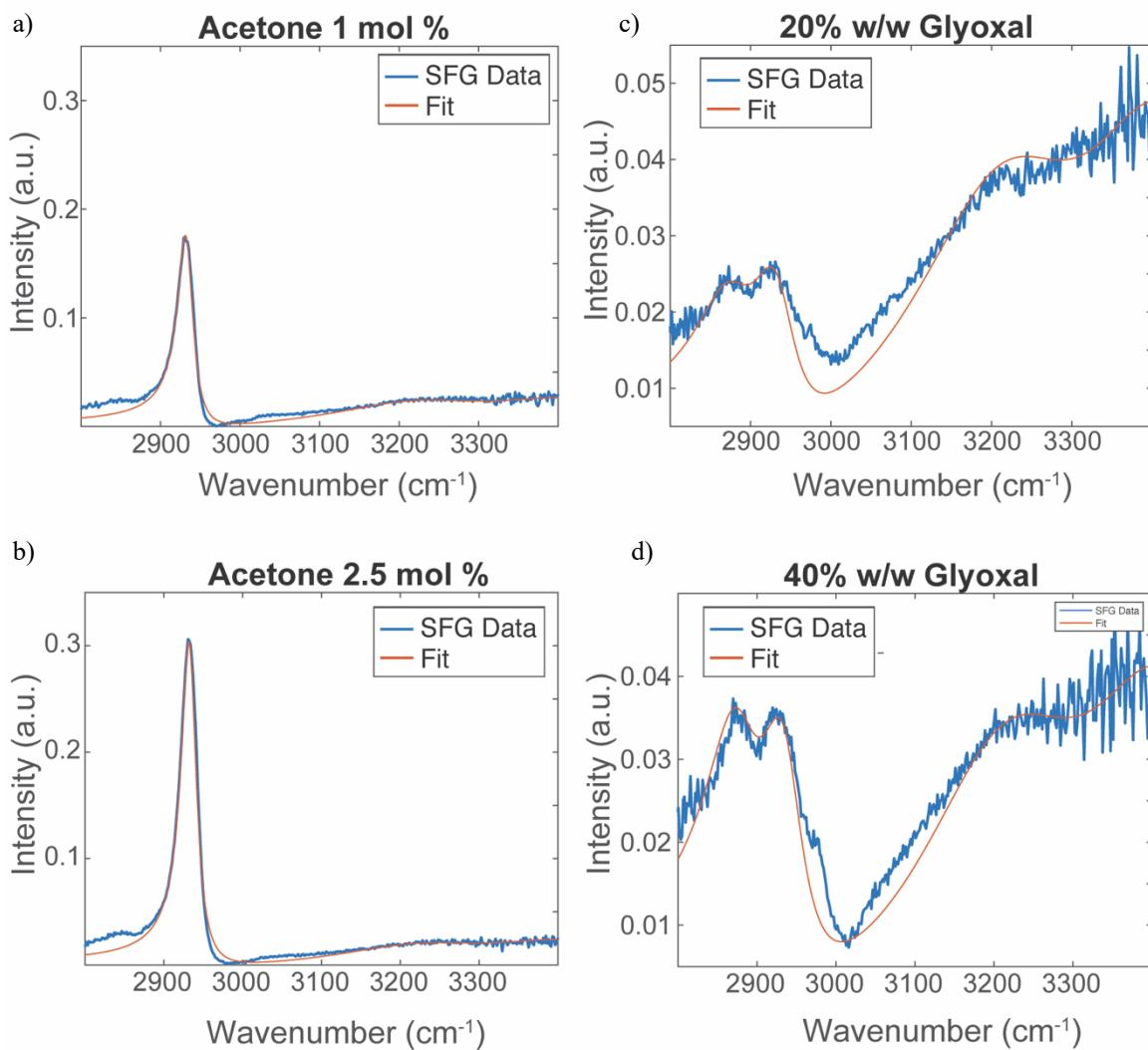
Figure 3.3. SFG spectra of acetone (a and b) and glyoxal (c and d) solutions in the CH stretch region (blue) with fitting (red).
