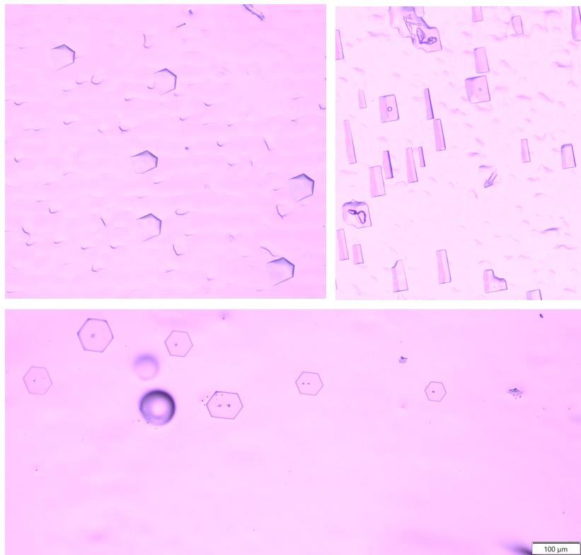
Figure 2.3. Etch pits of off axis basal plane (a), primary prism (b), and oriented basal (c) ice.
