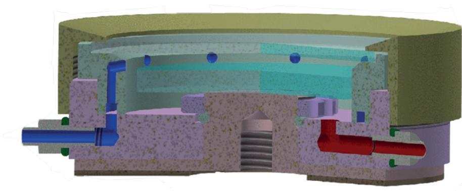
Figure 2.6. Diagram of flow cell and nitrogen flow over the ice.
