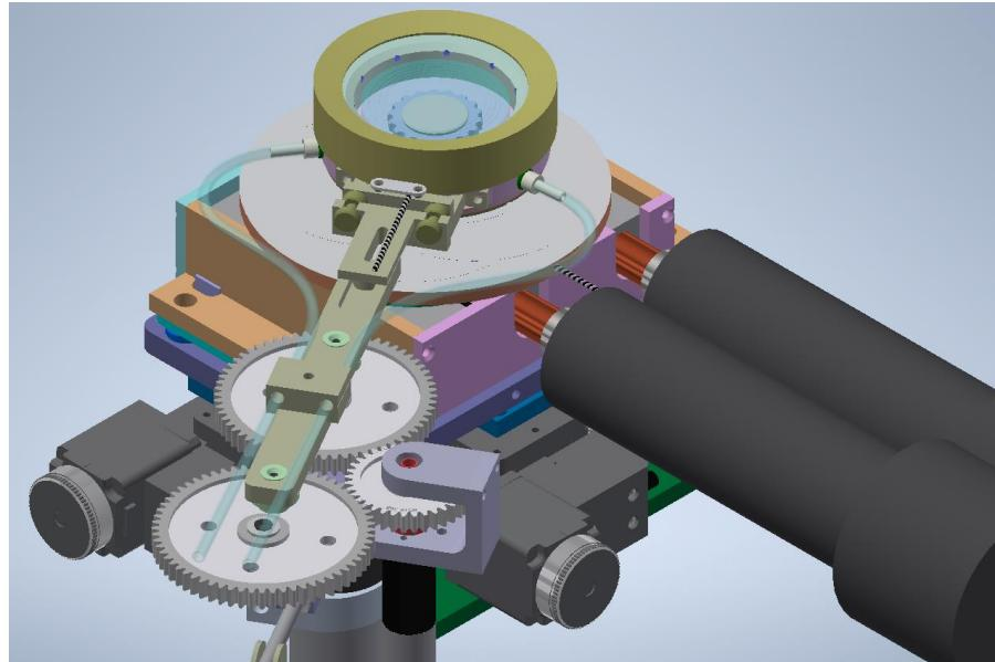
Figure 2.4. Diagram of flow cell attached to cooling stage.
