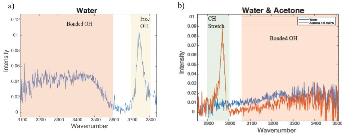
Figure 3.1. Vibrational SFG spectra of water in free OH (a) and CH stretch region (b).
