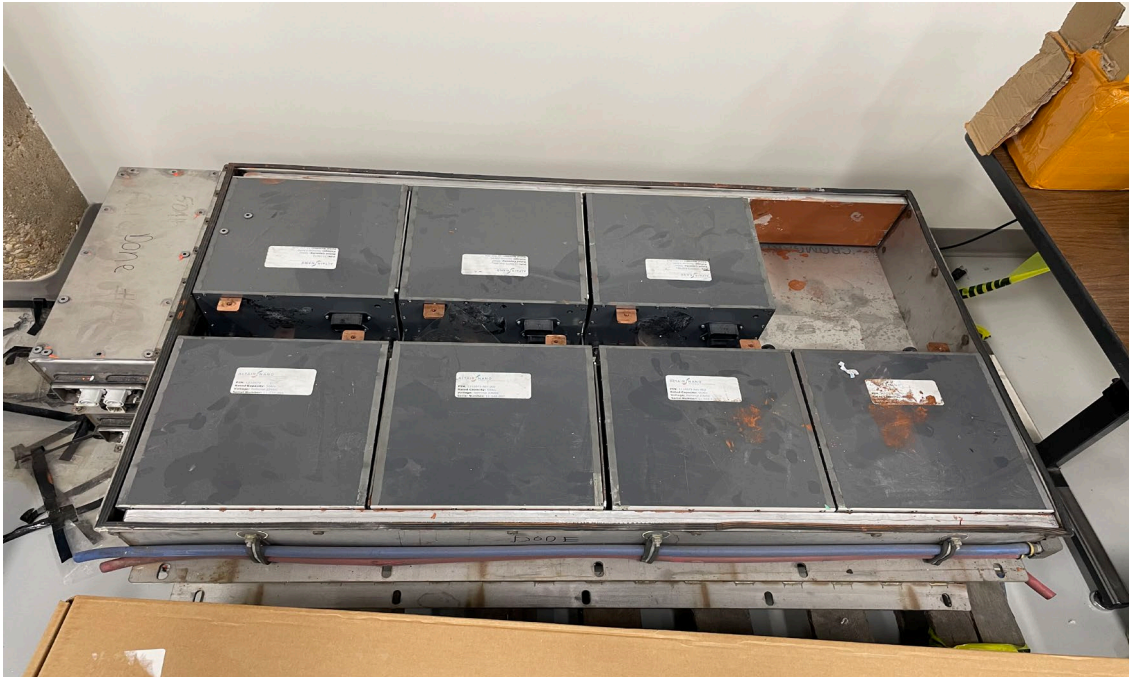
Figure 2.1. Original battery case donated by Proterra's electric bus.
