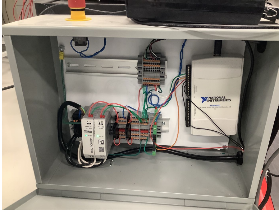
Figure 3.8. Data Acquisition (DAQ) setup.
