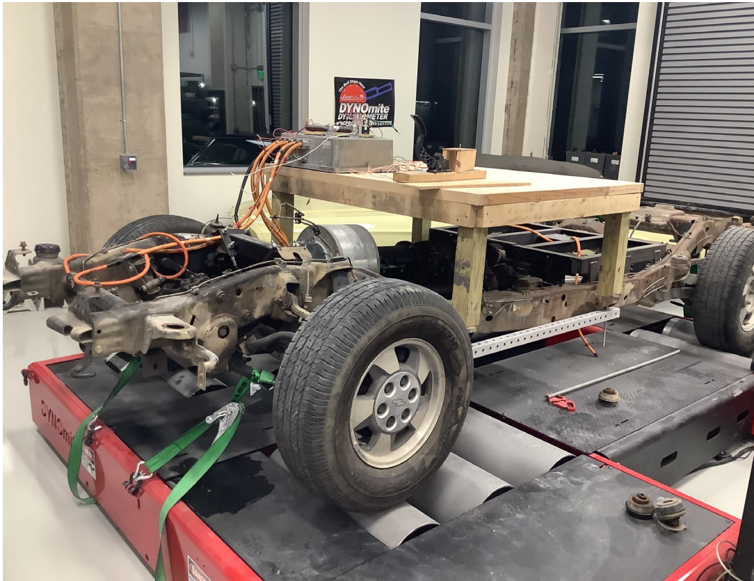
Figure 1.1. Converted all-electric Chevy Tahoe on the red and black Dynamometer.
