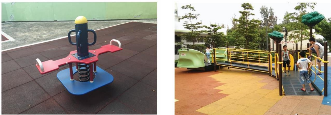
Figure 2.4. Comparison of accessible and inclusive seesaws. The accessible seesaw (left) does not differ much from traditional seesaws, but the inclusive seesaw allows independent entry and use by people who use mobility devices. From Siu et al., 2017. Photos are available for reprinting through a creative commons license.
