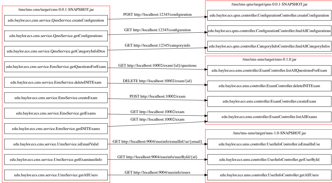
Figure 3.5. Inter microservice REST communications in TMS.
