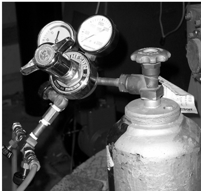
FIG.2.4 : The externally connected gas cylinder with the regulator.
